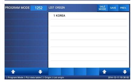
• Press Print Key to List Origins on screen. After Origins are listed on the screen, pressing the TEST key will print the Origins.
