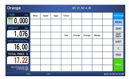
© Press the PRINT key. Markdown(STRIKE THROUGH) is printed on label as figure.
