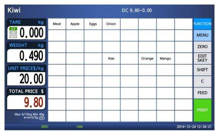
3 Place an item on the platter. In this case, discount is possible because the weight of item (0.526 kg)is greater than 1st target (0.500kg) therefore the total price is 10.26.
