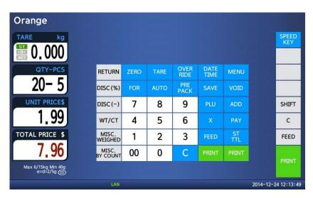
③ Press "PRINT" key to print a label and complete current transaction. This transaction(s) is saved in the sales record.
