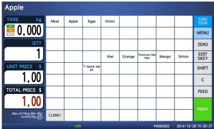
4 Place an item on the platter and press the V1 key.
